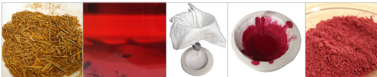
Figure 1 Reproduction of the making of brazilwood lake pigment.
