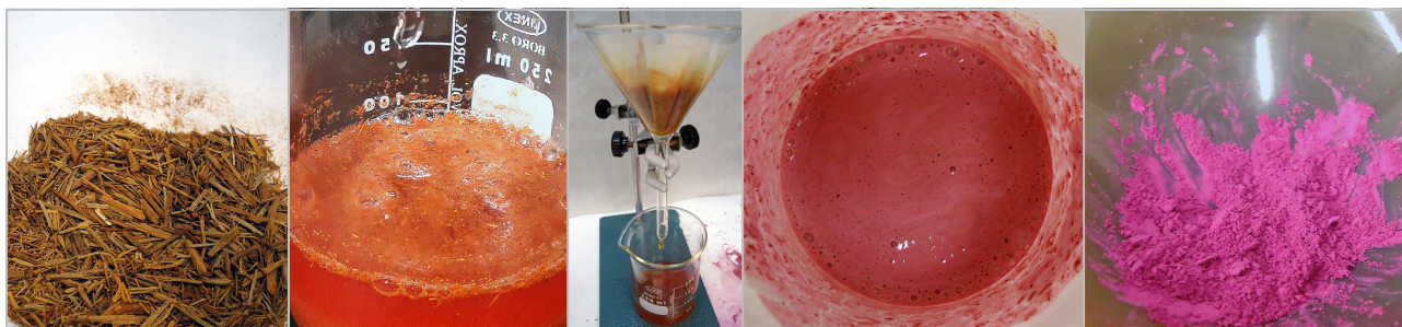
Figure 1 Reproduction of the making of brazilwood lake pigment.
