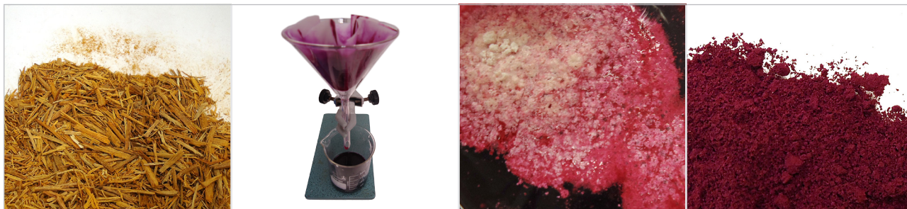
Figure 1 Reproduction of the making of brazilwood pigment lake.
